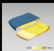
The seat is molded from urethane offering three different levels of firmness. The front of the chair uses a softer urethane for thigh comfort. The rear of the seat is made of a firmer cushion for greater support.
